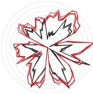
Figure 6a: Signatures of the wire samples captured by the NeOse Pro at 150°C.
