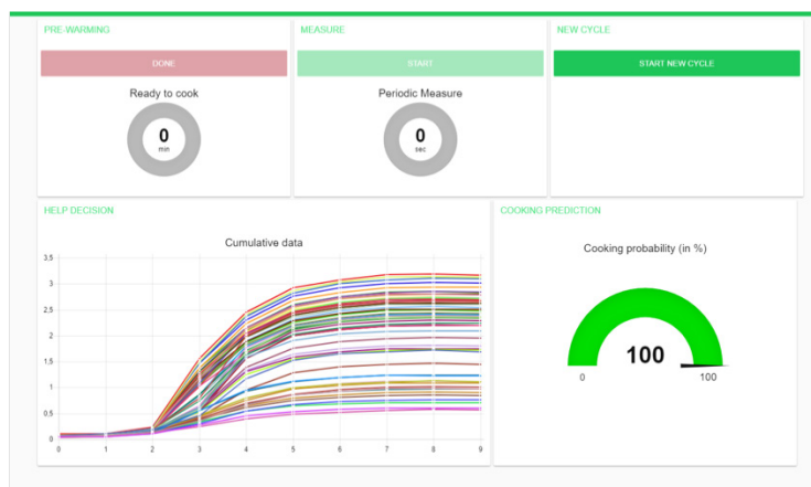
Figure 4: Basic software interface showing oven controls and odor data.
